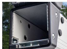
Pipe carrier liner
