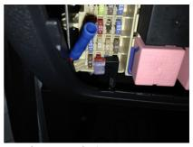
4. Insert fuse jumper into fuse box.
