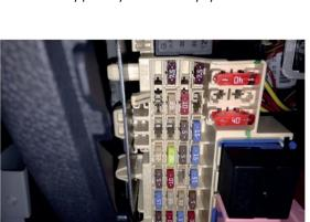
2. Open fuse box and remove selected fuse.
