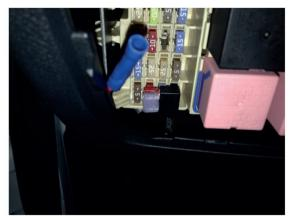
4. Insert fuse jumper into fuse box.
