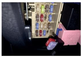
3. Place selected fuse in lower jumper terminal. Place 2A fuse, which supplies the ignition feed to the DC-DC charger, in top terminal. Be mindful of orientation
