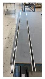
Prime rail and corresponding roof surface. Wait 10 minutes for the primer to dry.
